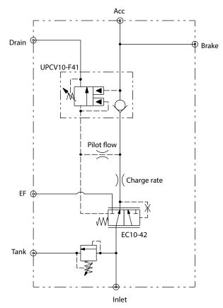
This circuit demonstrates accumulator charging as a priority function with a bypass type compensator. The UPCV pilots the EC while sensing the accumulator pressure. Orifices in the circuit control charging rate and pilot flow. The EC pilots downstream of the control orifice.
