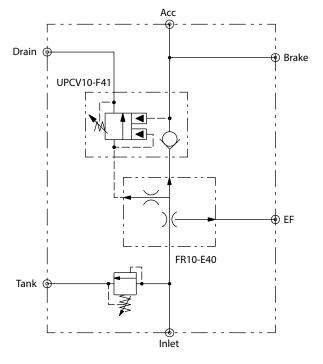
This circuit shows how you might apply the UPCV10-F41 to charge a brake accumulator. The UPCV pilots the FR while sensing the accumulator pressure. The valve cycles to maintain accumulator pressure within a specified range. The FR bypasses excess flow.
