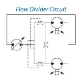
**Efficiency**: HydraForce makes very accurate flow dividers, but the accuracy relies on significant margin pressure. The margin pressure is a net energy waste. In addition, accuracy can suffer at low system flows.
