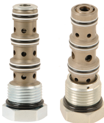
The FDxx-45 Flow Divider (right) is the recommended replacement for the FDxx-40, -41, and -42 flow dividers (left). It has a modified cage with larger ports in the center. The nose of the valve has a more durable tip as well.
