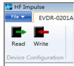
After the **Write** button has been clicked, *HF-Impulse* responds, asking to confirm download. A success message displays when complete.
