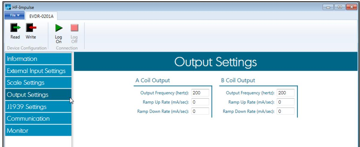
The *Output Settings* screen has sections for the A and B outputs. Each of these contain settings for output frequency, ramp up rate, and ramp down rate.
