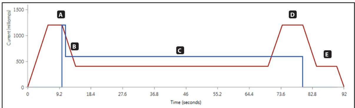
The ramp settings on the *Output Settings* screen cause the slopes in the chart. Be sure to allow enough time for the ramps. Otherwise the coils may not reach the intended amperage.
