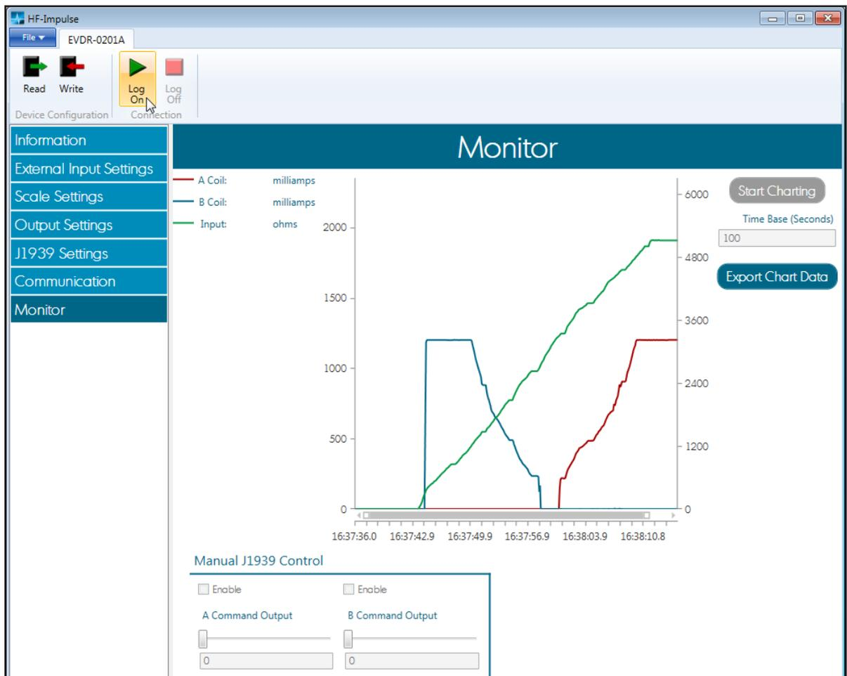
The chart area plots the *A Coil*, *B Coil*, and *Input* values over time. The Y axis on the left side is scaled from 0 to 2000 milliamps for the coil outputs. The Y axis on the right side is scaled in units based on the external input value. The X axis is scaled in time based on the entry in the *Time Base* box. Change *Time Base* as desired. *HF-Impulse* captures 10 samples per second.
